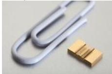
Fig. 24: Picture of a single emitter mounted on a CuW heatsink (screening submount).
